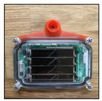
The larger knobbly bit of the ear tag fitting is always on the same side as the solar panel. This means that the solar panel is always facing away from the ear of the animal.
