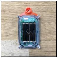
The shorter ear tag fitting allows the EarTraX unit to sit in the vertical plane.
